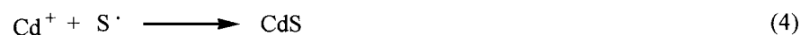
Scheme 2 Mechanism of the formation of CdS nanocomposites with \text{CS}_2 as the sulfur source.
